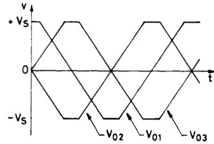
Fig. 2. Large signal oscillatory waveforms at the OA outputs.
