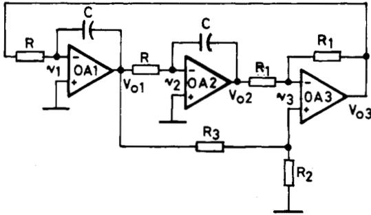
Fig. 1. KHN double integrator filter with input terminal grounded.
