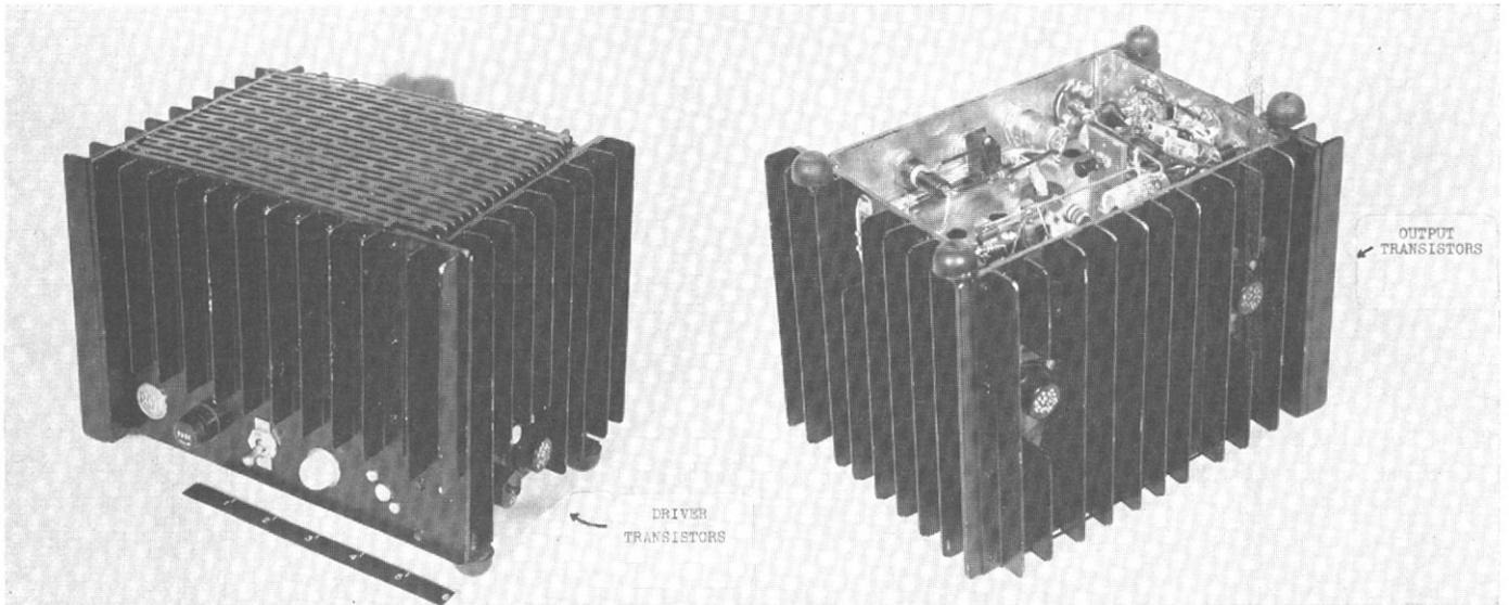
FIG. 1. 45-watt Quasi-complementary Amplifier. Left: Front view showing driver transistors. Right: Bottom view showing output transistors.
