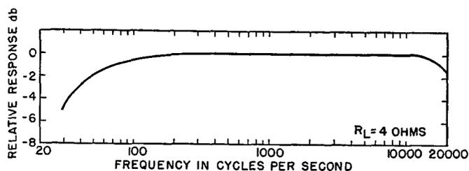
FIG. 7. Frequency response of 45-watt Series Amplifier.
