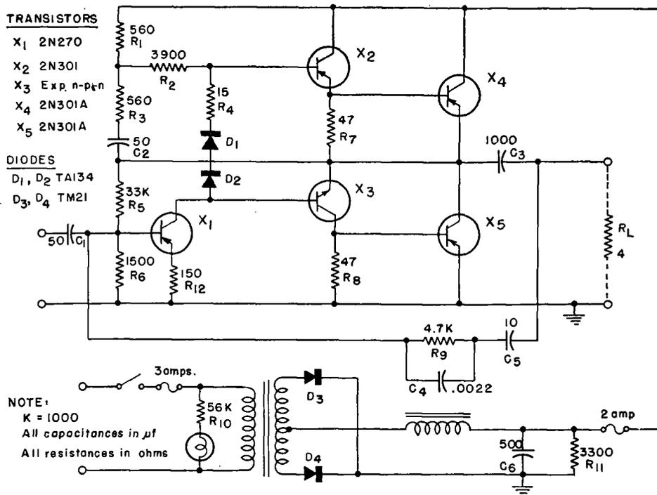
FIG. 2. Circuit diagram of 45-watt Quasi-complementary Amplifier.
