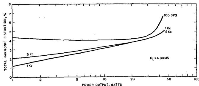
FIG. 6. Distortion vs. Power Output for 45-watt Series Amplifier.
