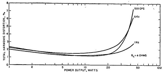
FIG. 3. Distortion vs. Power Output for 45-watt Quasi-complementary Amplifier.
