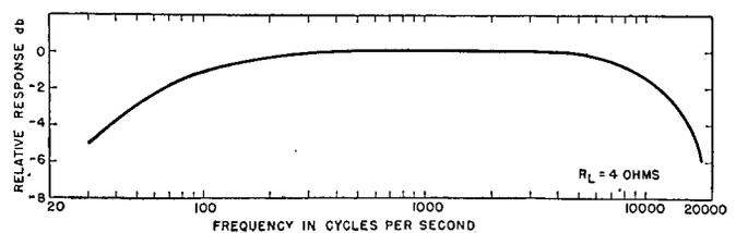
FIG. 4. Frequency response of 45-watt Quasi-complementary Amplifier.
