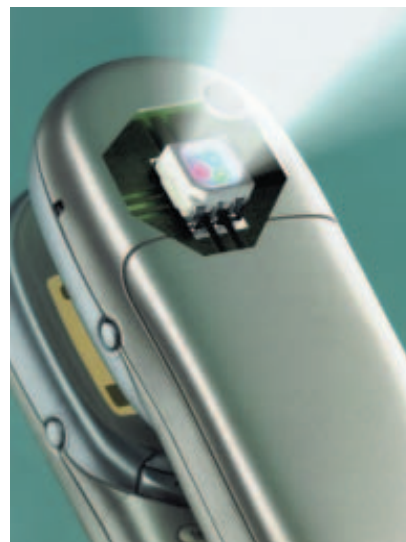
LEDs can replace conventional discharge lamps to provide the flash for mobile-phone cameras. Unlike discharge lamps, LEDs require no charge-up time (courtesy Osram).
